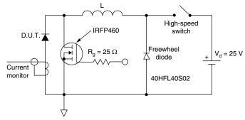
Fig. 6 - Unclamped Inductive Test Circuit
